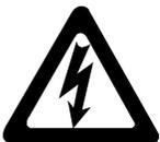
**ELECTROCUTION HAZARD**—High voltage is present inside electric boxes, motors, and many other components. Power switches on machine disable only control circuit power in certain boxes. You can be killed or seriously injured on contact with high voltage.
