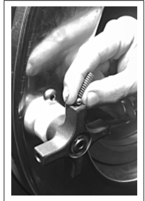
FIGURE 12 (MSSM0288AE) Inserting Ball and Spring in Handle Spoke
