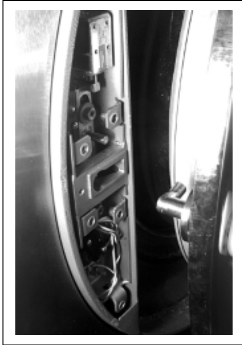
FIGURE 11 (MSSM0288AE) Shaft Finger Aligned with Locking Mechanism Notch (Cover removed for clarity)
