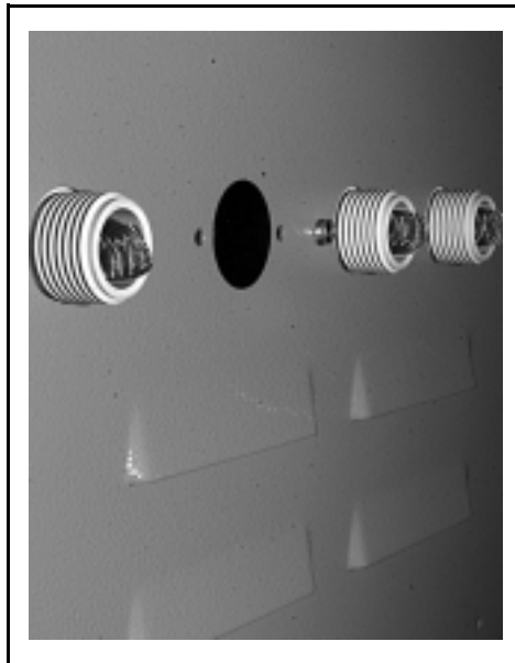
FIGURE 4 (MSSM0712AE) Inlet Valve Strainers
