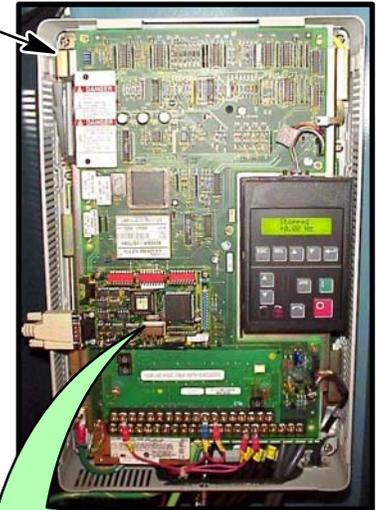
There are four communication LEDs located on the serial communication card. Under normal machine operations, the outside LEDs will be blinking. This is a visual indication that the controller is transmitting signals to the inverter, and that the inverter is responding to the signals. Only during a fault or error condition will one or both of the inner LEDs be illuminated. If an error or fault condition is discovered, call the Washex Service Department at 1-940-855-3990.
